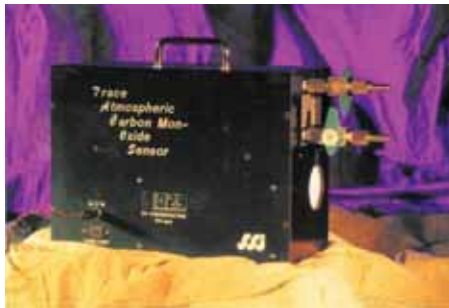
SSI gas measurement instruments: at top, open-path diode-laser sensor for HF installed in an aluminum pot room; at bottom, gas correlation sensor for carbon monoxide.
