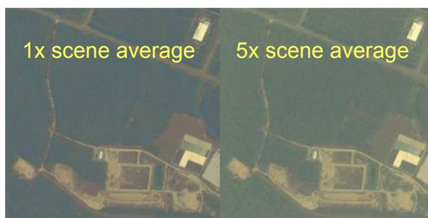
**Figure 7.** Effect of boundary region reflectance on the apparent reflectance of the Stennis scene. The sensor is at 20 km and the solar zenith angle is 30 deg. At left, the boundary region reflectance is taken as the scene average. At right, the boundary reflectance is 5x higher.
