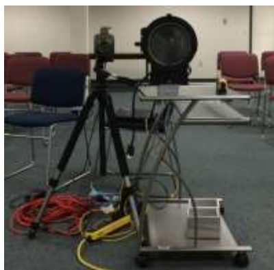
Figure 11. Phantom v7.1, 10 bit, well depth 80,000 electrons, and light as placed for this experiment.
