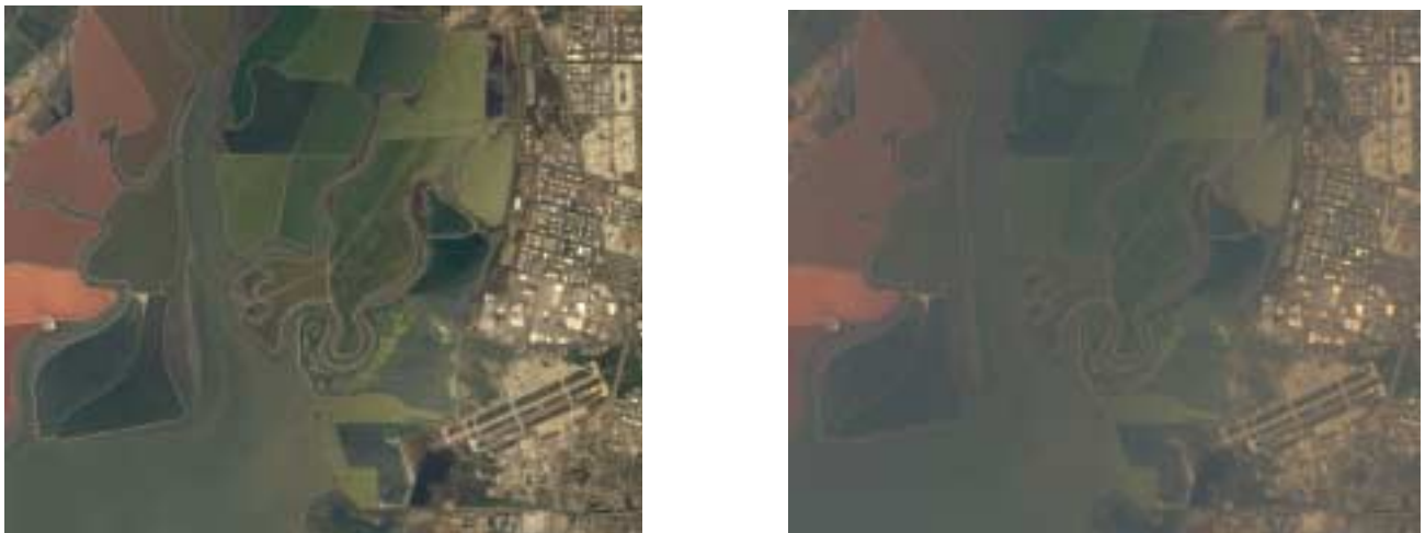
Figure 3. AVIRIS Moffett Field scene (left) and simulation with a 5 km visibility urban aerosol (right).
