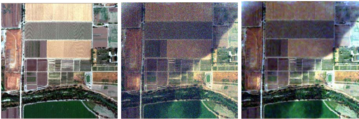
Fig. 8. Davis, CA hyperspectral scene simulations. At left, input surface reflectance; at center, MCScene apparent reflectance output; at right, the result after noise removal.
