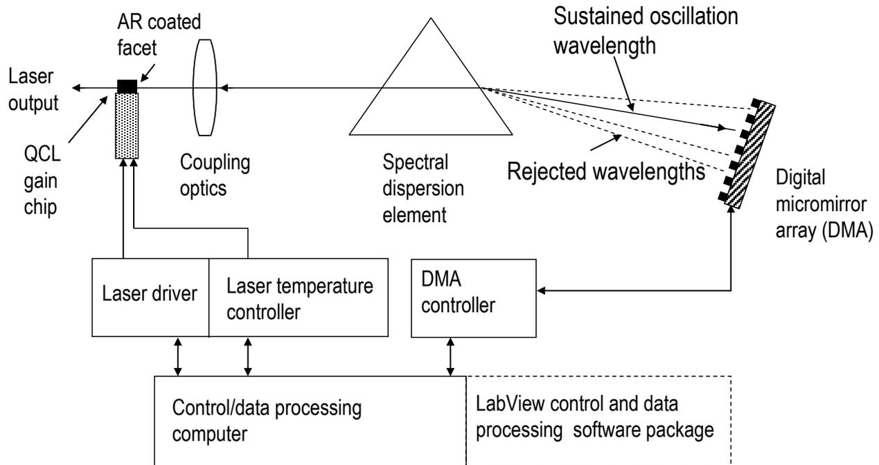
Figure 1. Digitally tunable quantum cascade laser concept.
