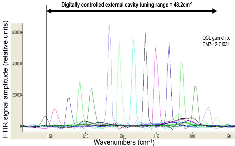
Figure 4 (b). The tuning curve of the CM7-12-CI0316 chip showing tunability between 1173.0cm<sup>-1</sup> and 1221.2cm<sup>-1</sup> (8.18μm to 8.52μm) spanning 48.2cm<sup>-1</sup> (0.34μm).
