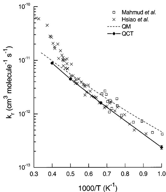
FIG. 1. Thermal rate constant for  $\text{O}+\text{HCl}(v=0)\rightarrow\text{OH}+\text{Cl}$  from 1000 to 3000 K.  $\square$ , Measurements of Ref. 3;  $\times$ , measurements of Ref. 2; ---, QM results of Ref. 15,  $-\blacklozenge-$ , present QCT-HB results.
