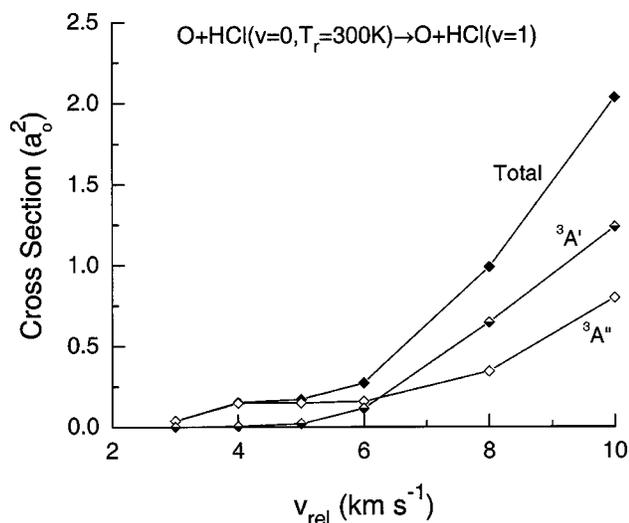
FIG. 10. Total and electronic state component collisional excitation cross sections vs relative collision velocity for the QCT-HB results for the transition  $\text{O} + \text{HCl}(v=0, T_r=300 \text{ K}) \rightarrow \text{HCl}(v'=1) + \text{Cl}$ .  $\blacklozenge$ , Total cross section;  $\diamond$ ,  ${}^3A''$  component;  $\blacklozenge$ ,  ${}^3A'$  component.
