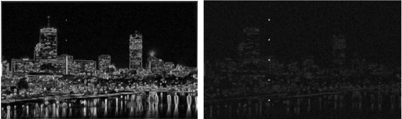
Fig. 3. Output detection images for random-wave signatures: unwhitened AC signal X at left, whitened signal X' at right.
