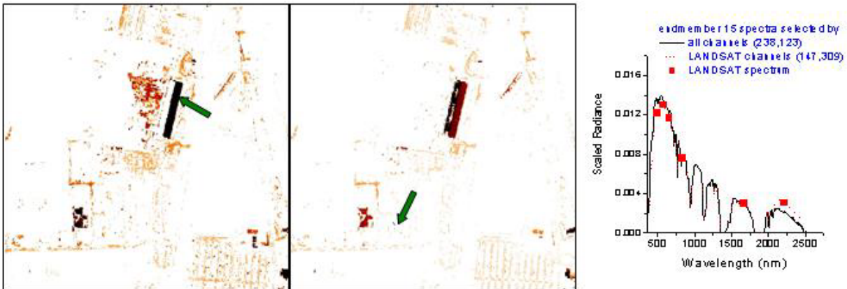
(a) (b) (c) Figure 17. Abundance maps derived from the full 224-channel calculations and the 6-channel calculations for endmember pairs (15) are in Figure 17a, 17b respectively. Arrows on the abundance maps point to pixel locations of the selected endmembers. The normalized radiance spectra of the endmember pairs are in Figure 17c.
