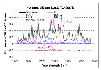
FIGURE 5. FIT TO SIMULATED SPECTRUM,  $\phi$ =0.6, SHOWING THE CONTRIBUTIONS OF THE FIRST TWO CO AND H<sub>2</sub>O BASIS SPECTRA.
