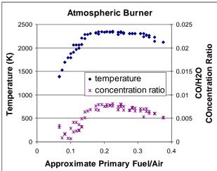
FIGURE 7. TEMPERATURE AND CONCENTRATION DATA DETERMINED FROM ATMOSPHERIC-PRESSURE FLAME SPECTRA. DATA ARE PLOTTED AS A FUNCTION OF THE MEASURED PRIMARY FUEL AIR RATIO BEFORE MIXING WITH AIR. TOP - OBSERVED RADIANT INTENSITIES OF  $\rm H_2O$  AND CO. BOTTOM - TEMPERATURES AND CONCENTRATION RATIOS.
