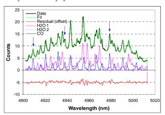
FIGURE 9. COMBUSTOR SPECTRA WITH LARGEST CO CONTRIBUTION, IDLE WITH PILOT FLAME. BLUE ARROWS MARK WELL RESOLVED CO FEATURES.
