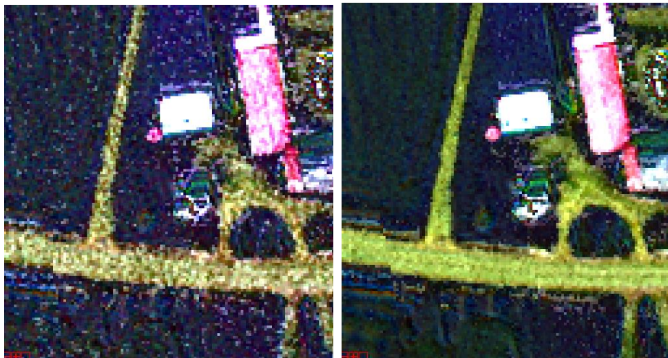
Figure 2. False color detail images of reflectance (red = 8.5 \mu\text{m} , green = 9.5 \mu\text{m} , blue = 10.5 \mu\text{m} ), from FLAASH-IR processing of a Hyper-Cam LW mosaic of farmland near Quebec City. At left, without de-noising; at right, with de-noising.
