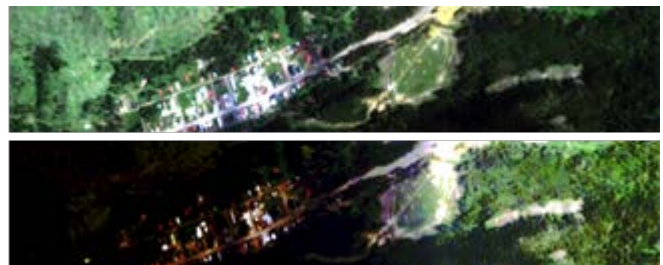
Figure 5. RGB radiance images simulated by MCScene for a subset of the RIT Target Detection Self-Test scene for cloud-free (top) and a 2/3 cloud shadowed scene (bottom).
