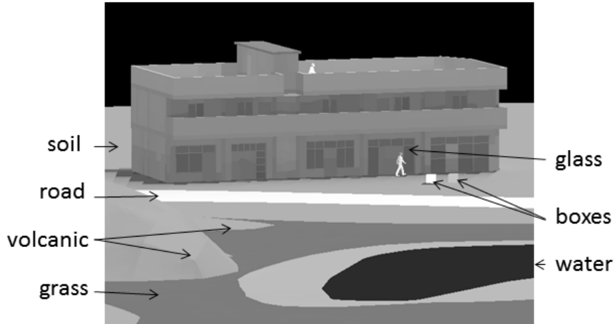
Figure 1. Temperature image of the MuSES scene. Grayscale corresponds to a temperature range of 290 K (black) to 320 K (white).
