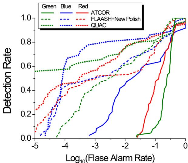
**Figure 6.** ROC curves for the large sunlit green, blue and red targets using three different atmospheric compensation techniques.
