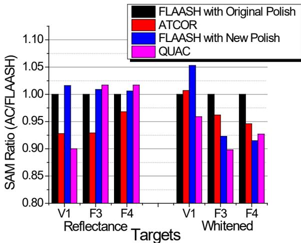
**Figure 3.** Spectral angle results for different atmospheric compensation approaches normalized to FLAASH SA result.
