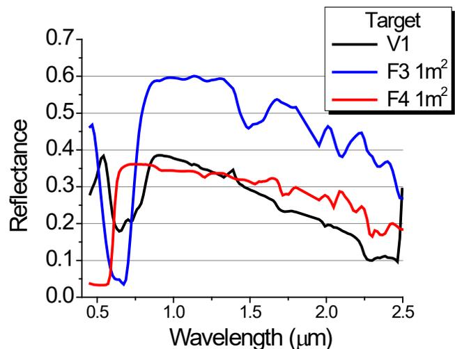
Figure 2. Spectral reflectance for targets used in this study.
