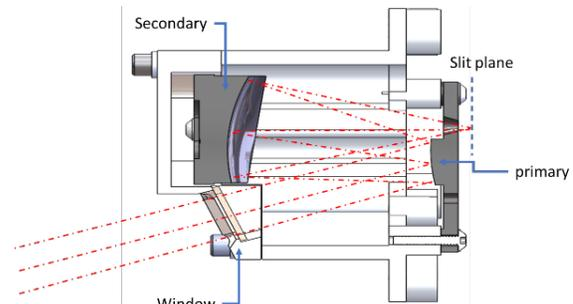
**Figure 6.** Cross section of fore-Optic telescope.
