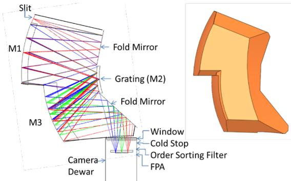
**Figure 5.** Ray Trace of spectrograph, Camera, and OSF.
