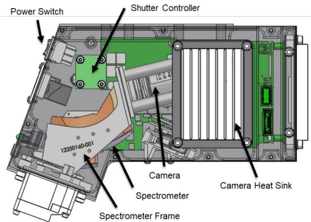
Figure 2. Cross sections of sensor flight package.
