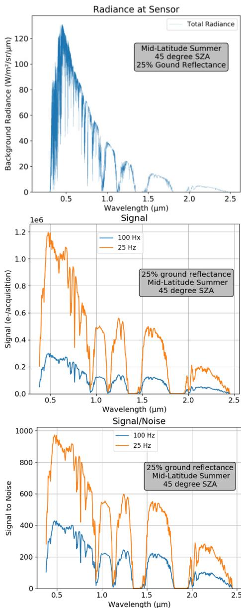
Figure 7. Predicted signal and SNR for a standard scene
