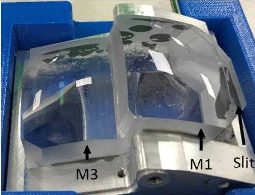
**Figure 4.** Partially completed spectrograph block. The top surface shows M3, M1, and the slit plane (left to right).
